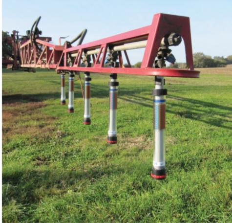
NOTE: Faster measurements can be obtained by using several FlowChecks at the same time placed at different sections along the boom. Always use clean water when undertaking the flow test and ensure suitable PPE is worn at all times.
